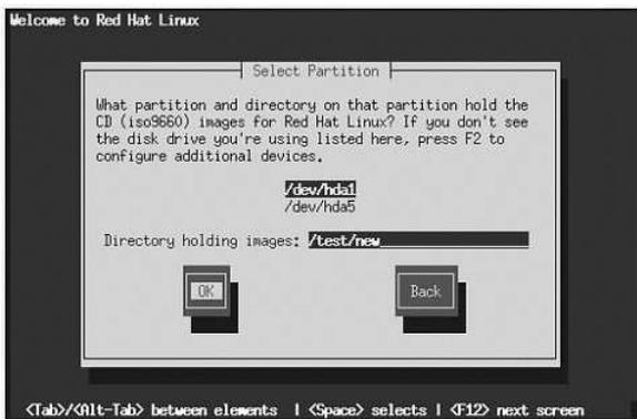
**Figure 3-3. Selecting Partition Dialog for Hard Drive Installation**
