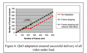
started the video running. After 60 seconds, we applied a load to the network link for 60 seconds, then removed the load. After another 180 seconds, 300 seconds in all, the experiment terminated. The data collector recorded each MPEG I frame (2 per second, 600 in all) that was sent from the sender, and each that was received at the receiver, and the time elapsed from send to receive.
