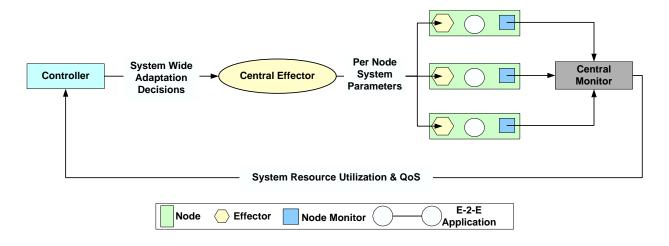
Figure 9: RACE's Feedback Control Loop
