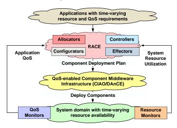
Figure 1: A Resource Allocation and Control Engine (RACE) for Open DRE Systems
