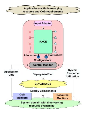
Figure 4: Detailed Design of RACE
