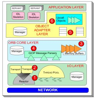
Figure 1. Layered CORBA Request Processing
