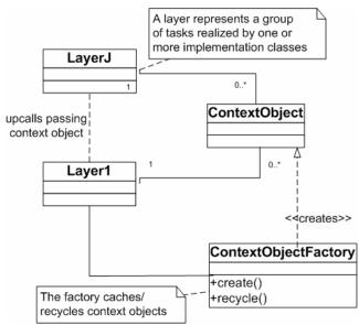
Figure 2. Structure of Context Object Pattern
