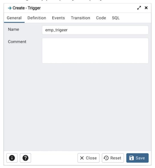
Use the fields in the *General* tab to identify the trigger:
