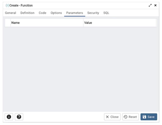
Use the fields in the *Parameters* tab to specify settings that will be applied when the function is invoked. Click the *Add* icon (+) to add a *NamelValue* field in the table.
