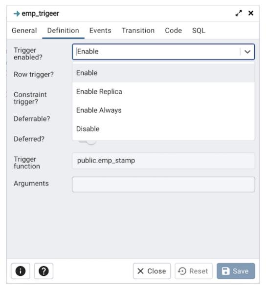
• *Trigger enabled* field is available in trigger dialog once the trigger is created. You can select one of the four options available.
