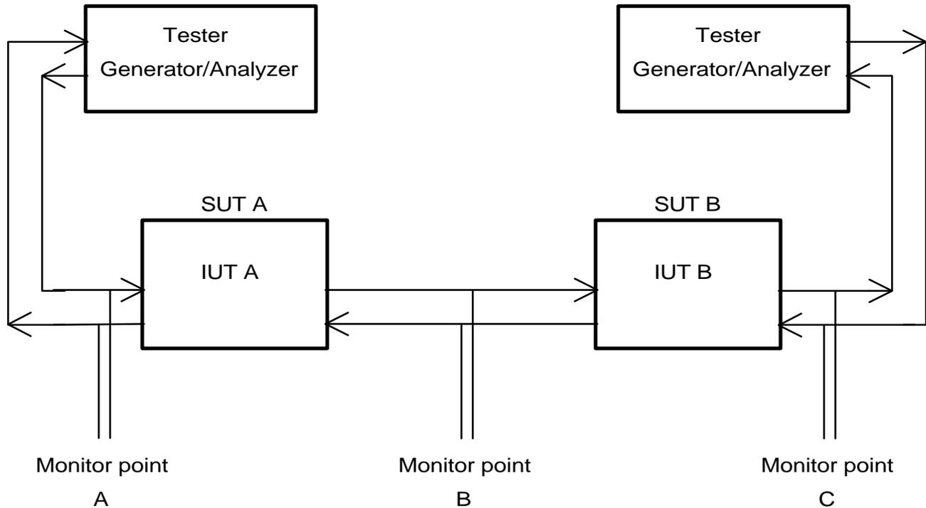
Figure 6.5: Generic Testing Configuration for Interoperability Testing
