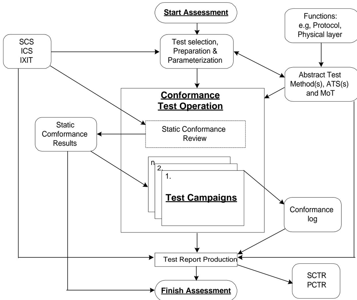
Figure 4.2: Conformance Assessment Process Model
