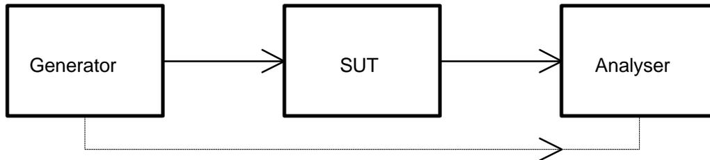
**Figure 5.1: Generic Test Configuration for Performance Testing**
