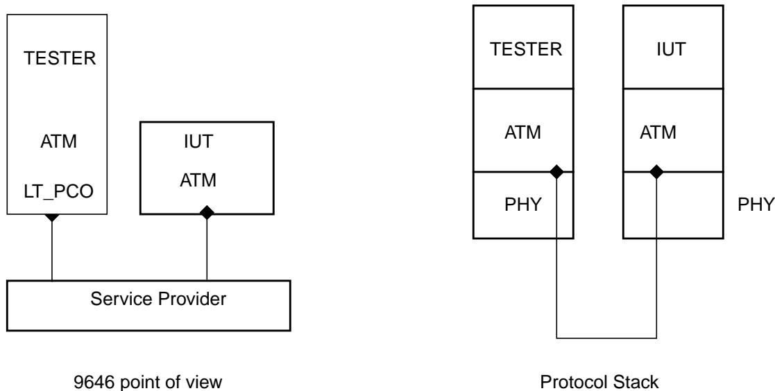
Figure 1. Configuration for testing of an End System.
