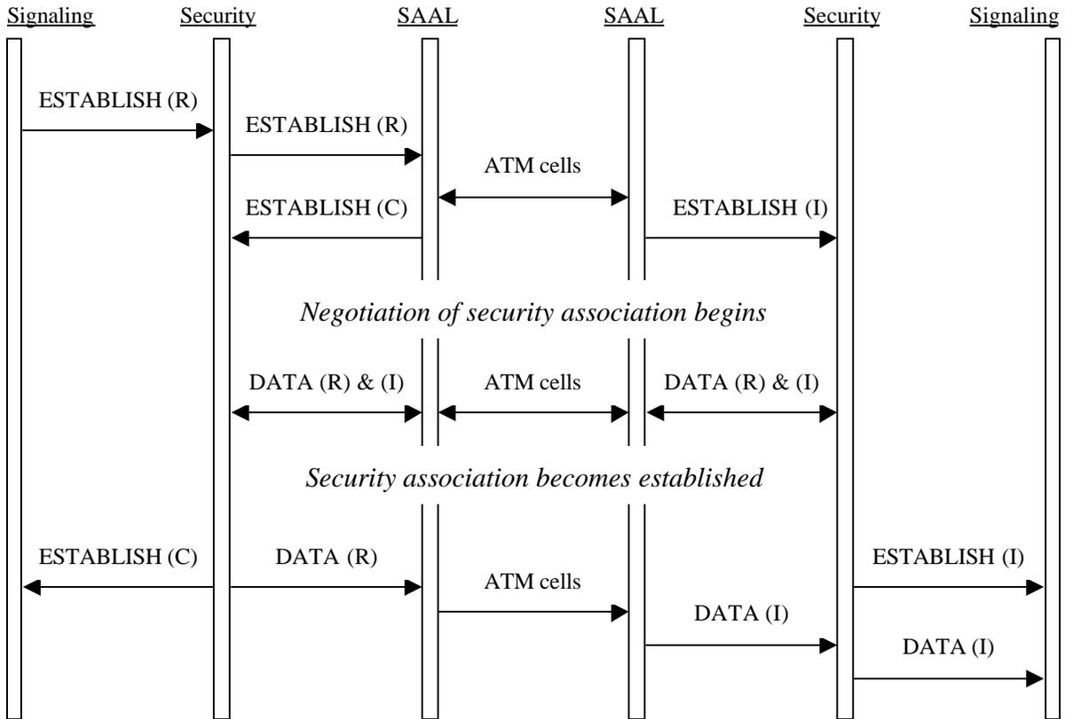
**Figure A-2: Connection Establishment With Data Transfer.**
