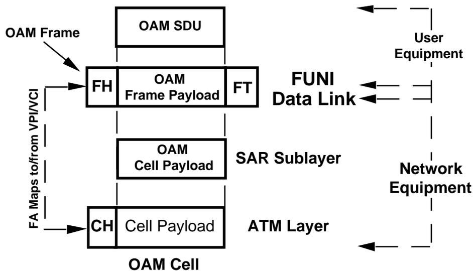
**Figure 5.1 Cell-to-Frame Mapping of Management Cells**
