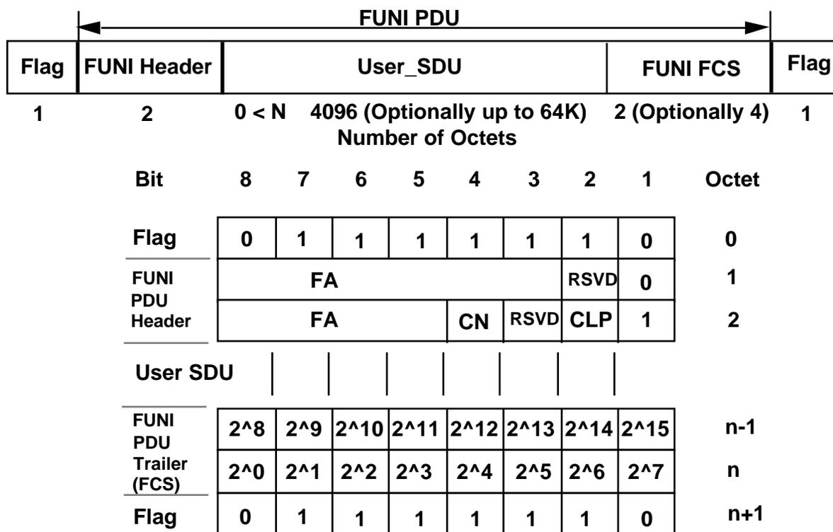
**RSVD** **Reserved** for interface management. These bits are set to 0 unless the frame is used for management per Section 5.2 below.
