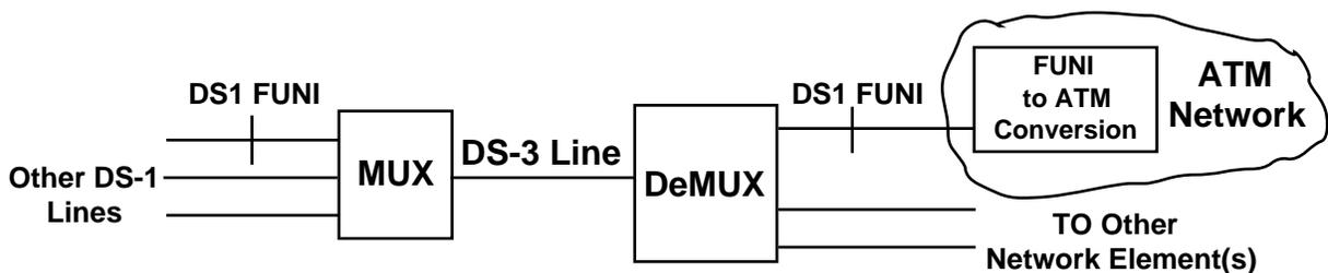
Figure 2.2a Example of Multiplexing/Grooming a DS-1 FUNI
