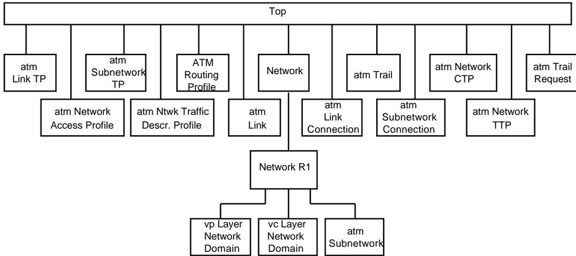
**Figure 2 Inheritance Diagram**
