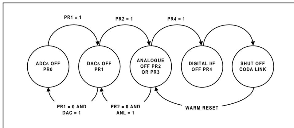
**Figure 14 The WM9704Q Powerdown/Flow with Analogue Still Alive**
