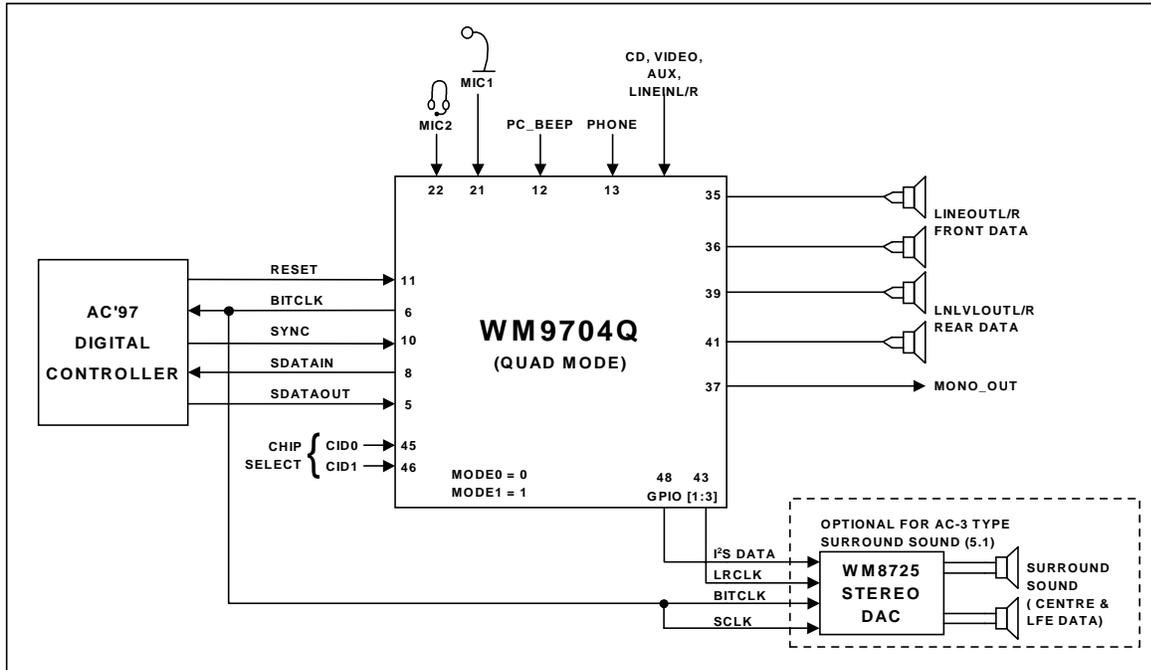
Figure 7 WM9704Q in Typical Quad Mode Application
