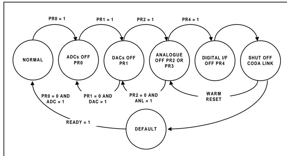
**Figure 13 An Example of the WM9704Q Powerdown/Powerup Flow**
