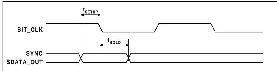
Figure 5 Data Setup and Hold (50pF External Load)
