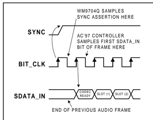
Figure 12 Start of an Audio Input Frame
